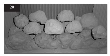
5.14 Place the centre rear small coal in the recess behind the large centre coal, Diagram 21
