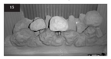
5.9 Place the front right medium coal on the front coals and against the flame baffle, Diagram 16.
