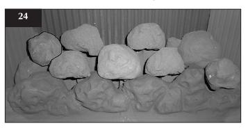
8.17 Place the centre rear small coal in the recess behind the large centre coal, Diagram 25
