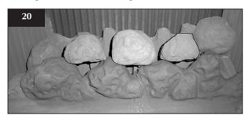
8.13 Place the rear left medium coal in the recess behind the front row of coals, resting on the rear panel, Diagram 21.
