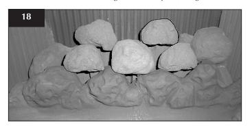
5.12 Place the right hand small coal in the recess between the flame baffle and the front coal, Diagram 19
