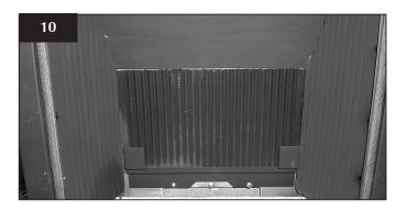
5.4 Position the flame baffle centrally on the tray and ensure the stepped lower edge engages against the rear edge of the burner skin, Diagram 11
