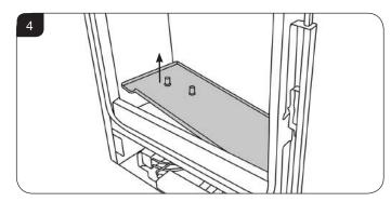
4.3 Slide the burner tray fully to the left and remove through the front of the firebox, see Diagram 4.
