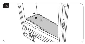
4b.8 Slide the burner tray fully to the left and remove through the front of the firebox, see Diagram 18.
