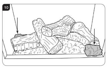
6.8 Spread a liberal amount of the Embaglow fibres provided on the sections highlighted, see Diagram 11.
