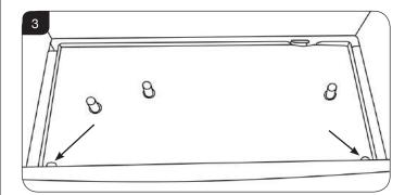
4.2 Lift the left hand side of the burner tray, before lifting the right hand side, see Diagram 4.
