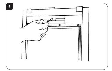
1.2 If the appliance spills, run for a further 10 minutes and re-check.
