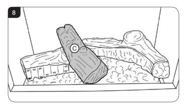
6.6 Log D fits onto the locating pin and rests on Log B, see Diagram 9.
