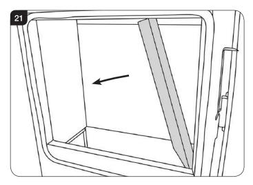
12.5 To remove the Left Hand liner first tilt inwards towards the centre of the firebox before lifting up and pulling out through the front of the firebox, see Diagram 21.
