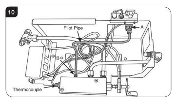
7.5 Replace with a new pilot assembly and check the spark gap, see Diagram 11.
