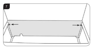
4a.9 Remove the 2 knockout holes on the rear of the box using a sharp hammer blow, see Diagram 8.
