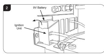
3.2 Remove the old battery and replace with a new high quality (Duracell or similar) 9V battery.
