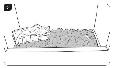
6.4 Log B is positioned on the right hand locating pin, and rests against the back liner, see Diagram 7.
