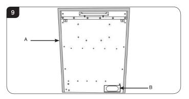
4a.11 Gas pipe entry must come through the rear of the box on the right-hand side. The rubber seal must be cut using a sharp knife to allow the isolating elbow to pass through it. Ensure the rubber is not damaged when doing this, see Diagram 8, Arrow B.
