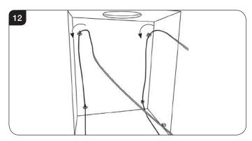
4a.15 Thread the ends through the holes in the lower back of the firebox. Pass the gas supply pipe through the hole in the rubber seal and push the appliance into place.
