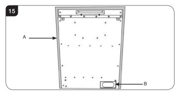
4b.3 Place the firebox centrally in the opening and mark the positions of the 4 fixing holes. Drill the holes and insert the 4 expansion plugs, see Diagram 16.
