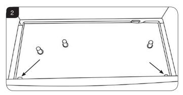
4a.2 Lift the left hand side of the burner tray to disengage from the injector, before lifting the right hand side, see Diagram 3.
