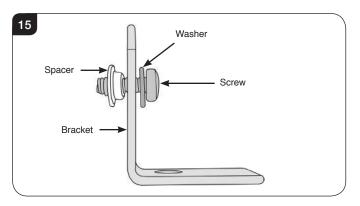
When replacing ensure that the components are assembled in the same order.
