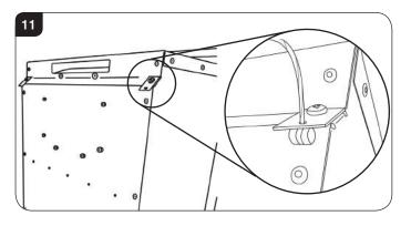
4a.14 Pass the cables vertically through the 2 sets of eyebolts, see Diagram 12.
