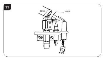
7.6 After reassembly check for gas soundness and carry out a flame failure functional check as detailed in the Fault Finding chart, especially the time it takes for the mag unit to close.
