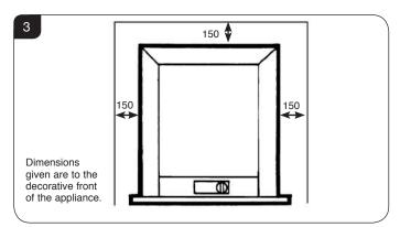
2.9 The maximum depth of combustible shelf is 150mm at a minimum height of 150mm above the decorative front. Refer to the appropriate Frame Instructions regarding additional wall strengthening for the frame.
