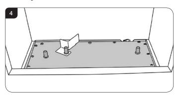
6.2 Place Log A in position on the 2 locating pins, see Diagram 5.
